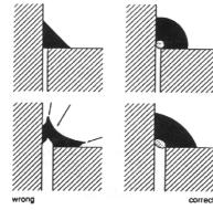
In corner joints too, the insertion of a release tape or backer rod is required, otherwise the sealant will fall during expansion of the joint.
